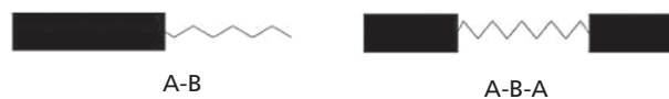
Figure 1 Schematic representation of PEGylated poly(lactide-co-glycolide)-poly(ethylene glycol) (PLGA-PEG) di-block (A-B) and PLGA-PEG-PLGA tri-block (A-B-A) copolymers. PEG (di-block): 5 kDa; PEG (tri-block): 6 kDa.
